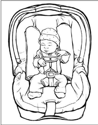
**Figure 4.** Car safety seat with a small cloth between crotch strap and infant, harness clip positioned at the center of the chest and at the level of the infant's armpits, and blanket rolls on both sides of the infant.
