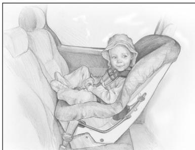
Figure 3. Convertible car safety seat used rear-facing.
